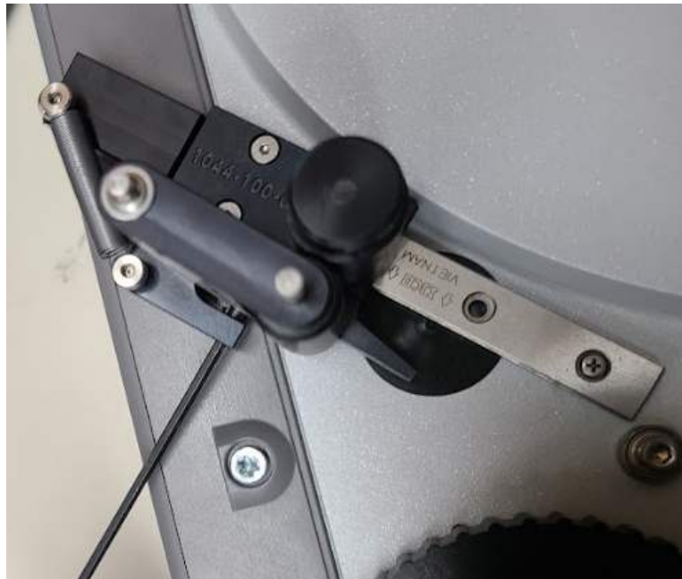
Figure 3. Adjustment screw, 2mm wrench.
