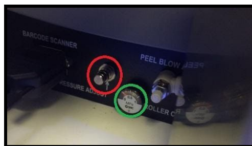
Figure 1. Roller Pressure Adjust Screw and Gauge
