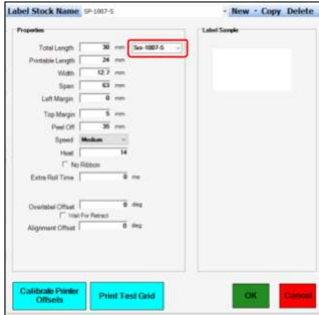
Figure 4. (SciPrintVX Software v 2.5) - In SciPrintVX software version 2.5, a dropdown list next to the Total Length field contains all Scinomix Label Kit part#s. Selecting the appropriate label part# will auto-populate the label characteristics.
