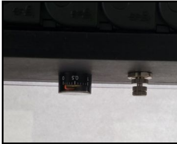
Figure 2. Gripper pressure gauge and pressure adjust flow controller screw
