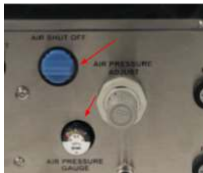
Figure 1. Air Shut Off valve and Air Pressure Gauge
